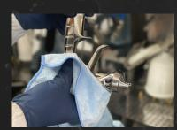
Remove the trigger clamp from the spray gun and 4 blow off the cleaning fluid from the spray gun. Meanwhile, leave the compressed air coupling connected and do not pull the trigger of the spray gun.
