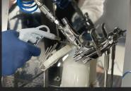
Open the spray gun with the trigger clamp. 3 Close washroom door and set timer to 2-3 minutes.
